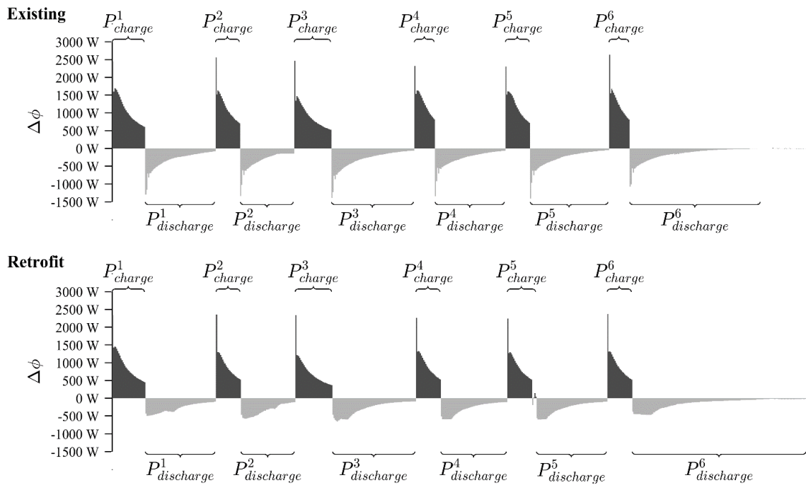
Fig. 12. Absolute shifting potential for the existing and retrofitted building using MPC setup b ).
