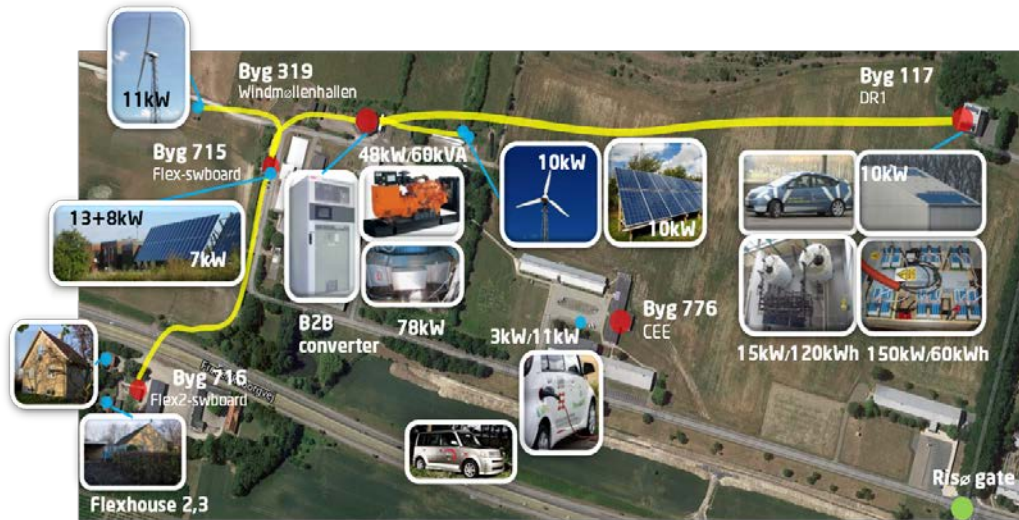
Figure 42: SYSLAB research facility with PV plants used for FRR service delivery.
