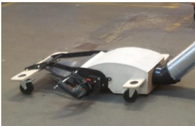
Figure 1.5.5.2. Function model of the new street nozzle with built-in-tank (white part to the right). Flow of debris is from left to right. The brush of the nozzle is driven by an electric power drill.
