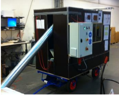
Test of fan, noise damping and suction mouth in Brøndby, December 2014
