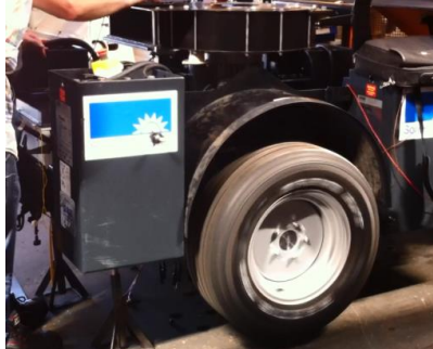
The wheels spinning for the first time after replacing the combustion engine with batteries
