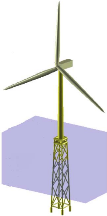
Figure 1: Illustration of the modeled turbine and jacket foundation.
