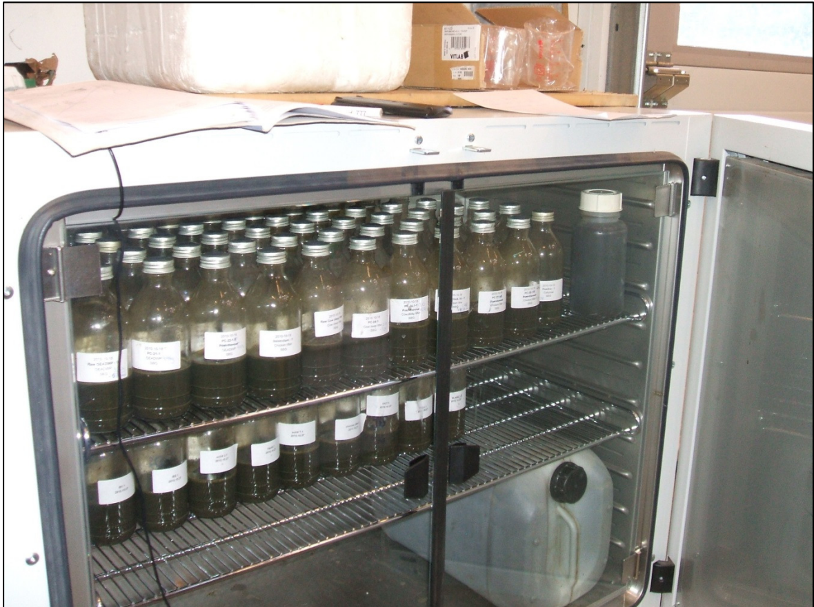
Figure 1. Batch test bottles in climate chamber for determination of biological methane potential.
