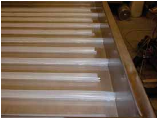
Fig. 4: Photos of the heat storage module with silicone pipes attached to the upper surface.
