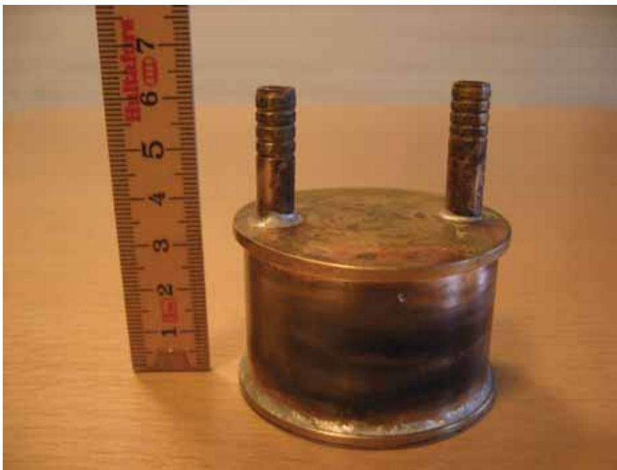
Figure 11: Brass tank with CO 2 used for starting the solidification.
