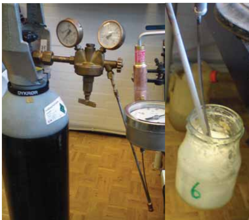
Fig. 2. Photos of the pressure container, the pressure reducing valve, the pipe system and the glass container.
