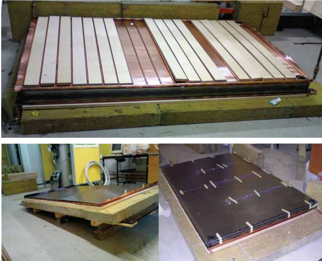
Fig. 8. Photos of the heat storage module.
