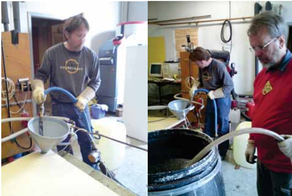
Fig. 5. Salt water mixture from a plastic tank pumped into a heat storage module.
