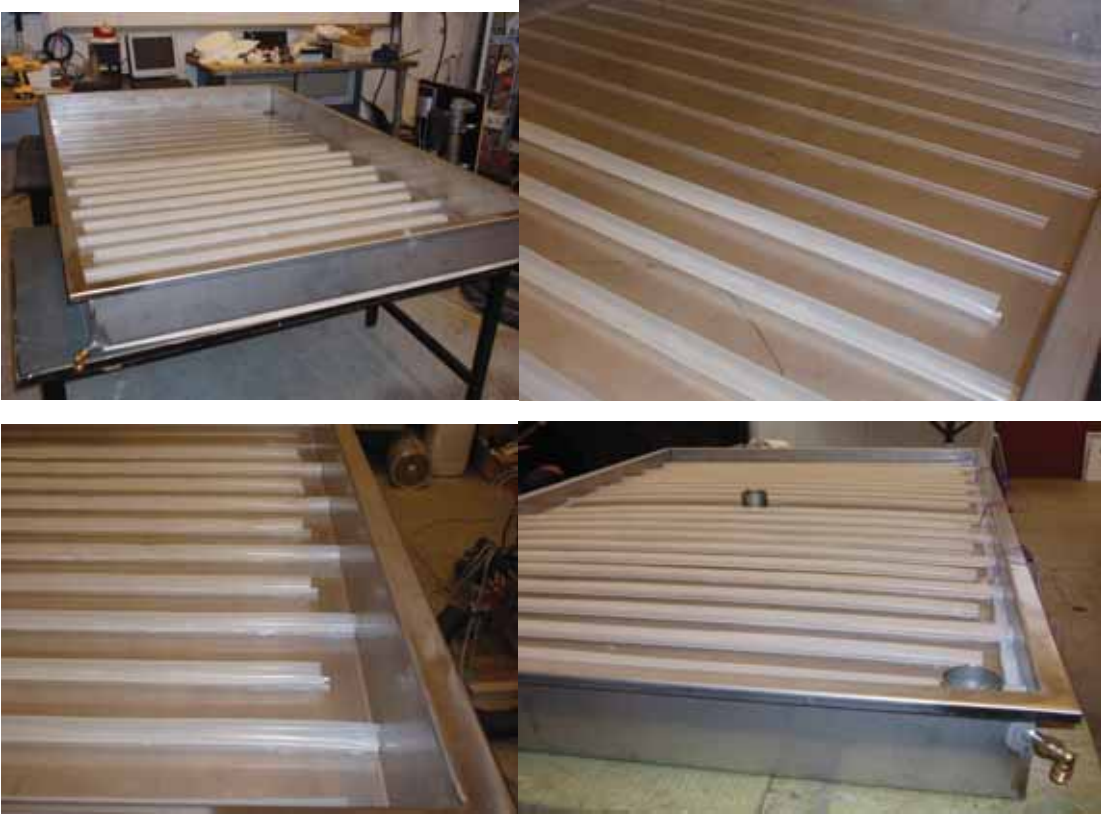
Figure 6: Photos of the first heat storage module with silicone pipes attached to the upper surface.
