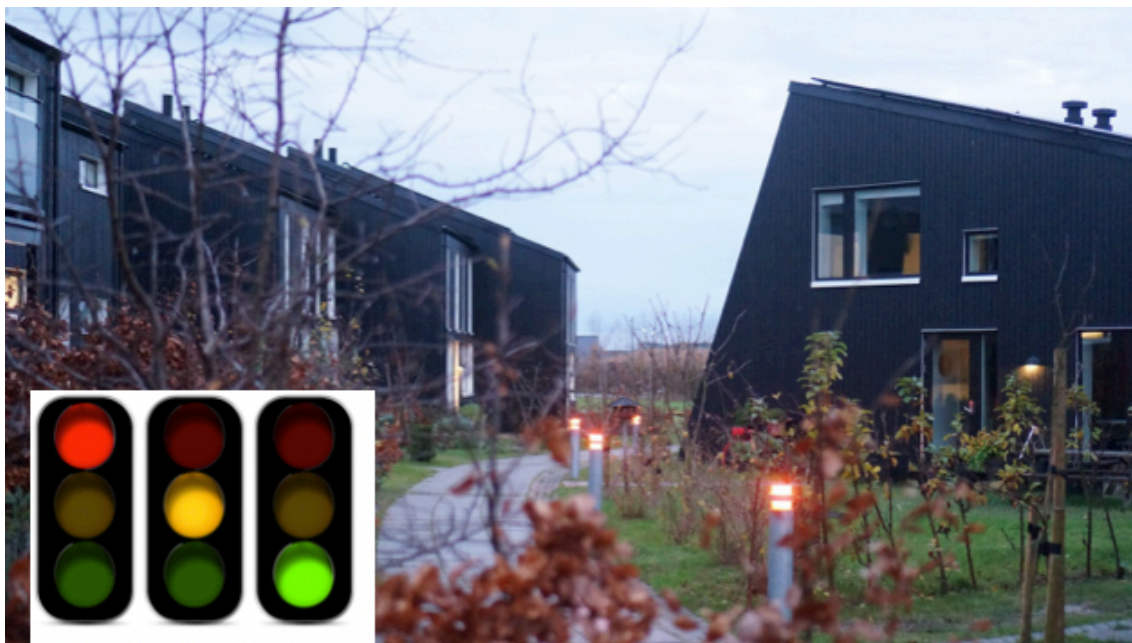
Figure 2 Colour changing pathway lights indicating the current CO2 intensity in the micro-grid
