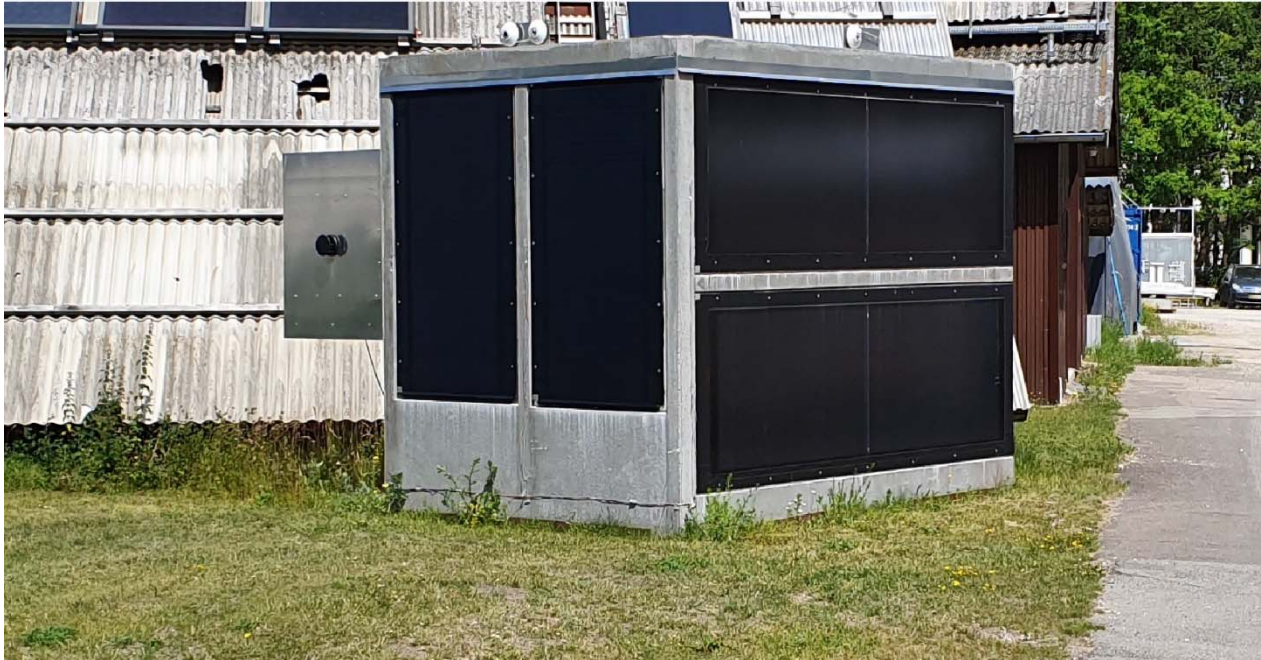
Figure 4.2(C)10 PVT-E modules encapsulated concrete wall On the right steel PV modules.
