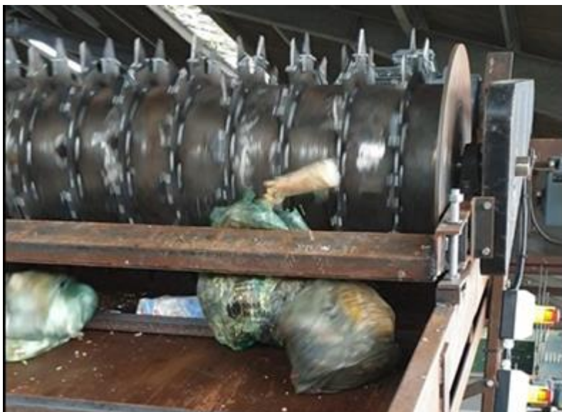
Figure 2: New bag opener with knives drum, before the safety casing was installed
