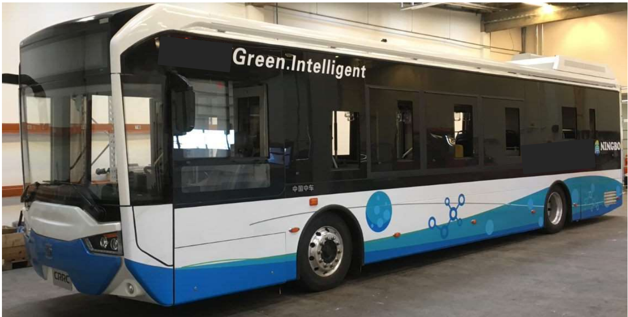
Figure 17: Fuel cell roof top box mounted on bus top.
