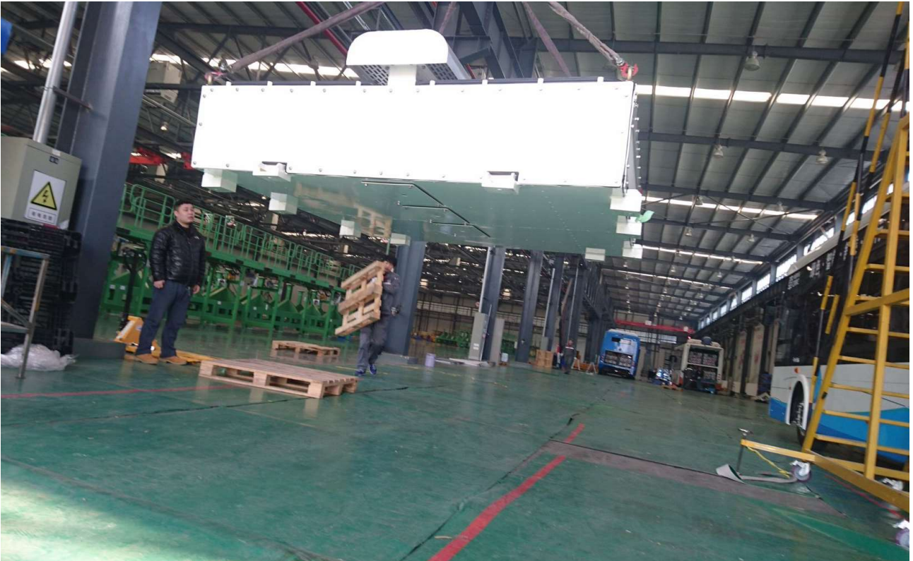
Figure 15: Fully assembled roof top box, ready for mounting on the electrical bus.
