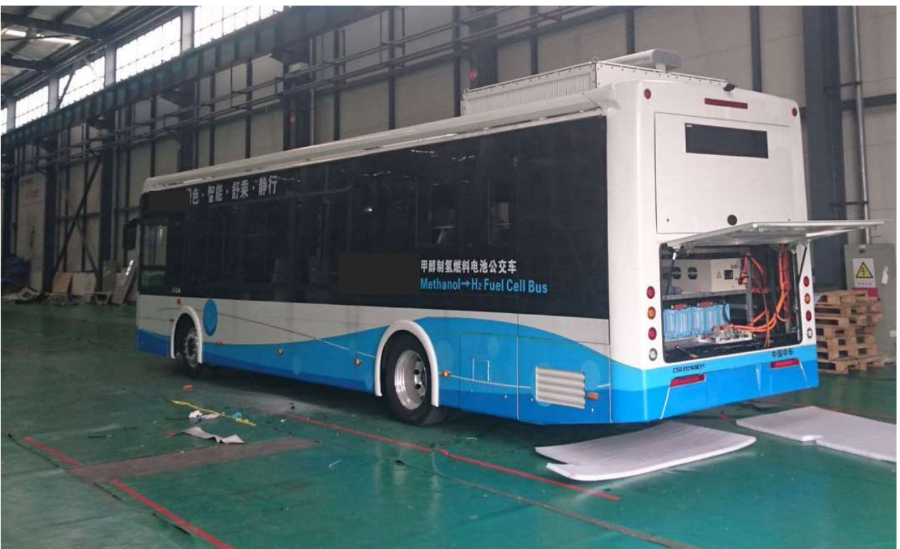
Figure 16: Fuel cell roof top box mounted on bus top.
