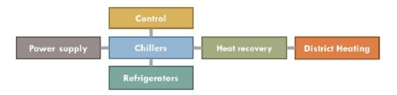
Figure 1: The figure 1 shows the chain components for recycling of surplus heat from chillers in supermarkets to the district heating system.
