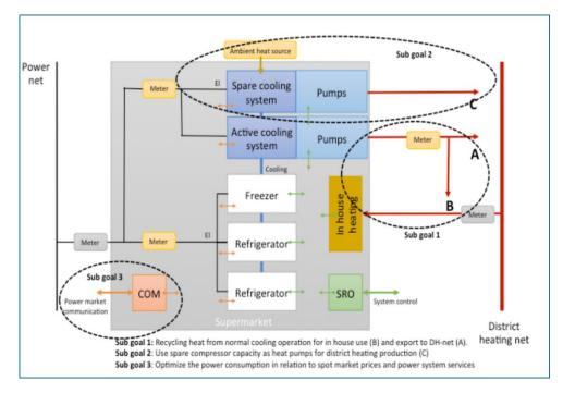
Figure 2: The figure 2 gives an overall view of possible solutions and sub-goals (models) for the recycling of surplus heat.
