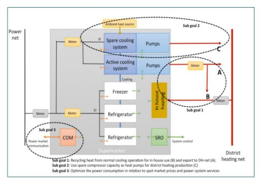
Figure 4: The figure 4 gives an overall view of possible solutions and sub-goals (models) for the recycling of surplus heat.
