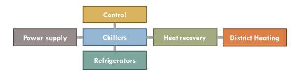
Figure 3: Elements of solutions of recycling of heat from the supermarket's refrigeration equipment for district heating purposes
