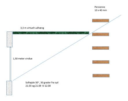
The shading system is very effective in cutting off direct solar radiation, in particular for south orientated windows. Above it is illustrated that the shading effect of the 10x40 mm blinds with a distance of 40 mm, this corresponds to the shading effect of a 3.3 m overhang, at spring or autumn equinox at 12.00 hours.
