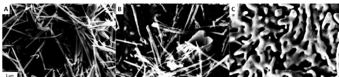
Figure 2: SEM micrographs of hydrothermally produced \text{NiMoO}_4 powders reduced in 5% \text{H}_2 and 3% \text{H}_2\text{O} (balance Ar) at 400 ^\circ\text{C} (A), 600 ^\circ\text{C} (B), and 800 ^\circ\text{C} (C).
