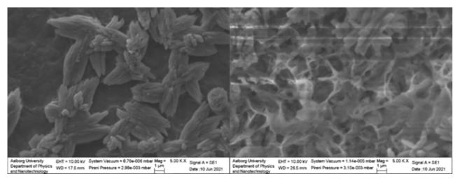
**Figure 1** – (Left) The needle like aragonite crystals on top of a porous brucite layer. (Right) Close up on the porous brucite layer.
