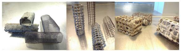
**Figure 2** - Cathodes electrified for 9 months and covered in mineral deposition, and cathodes not tested, first Hanstholm Installation.
