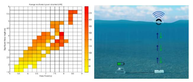
**Figure 4** – ResenWaves power curve validated in real sea environment (If). Resenwaves device with subsea hub (rg) \* <u>https://www.resenwaves.com/wave-energy-data-communications/#tech\_and\_testing</u>.
