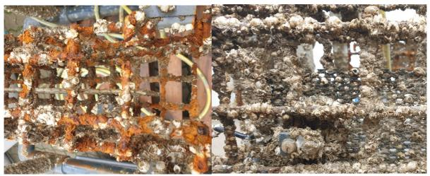
**Figure 7** - Control structure rusting away, from latest sea trials in Hanstholm harbor. Rg: electrified structure with mineral deposition highly colonized by marine organisms.
