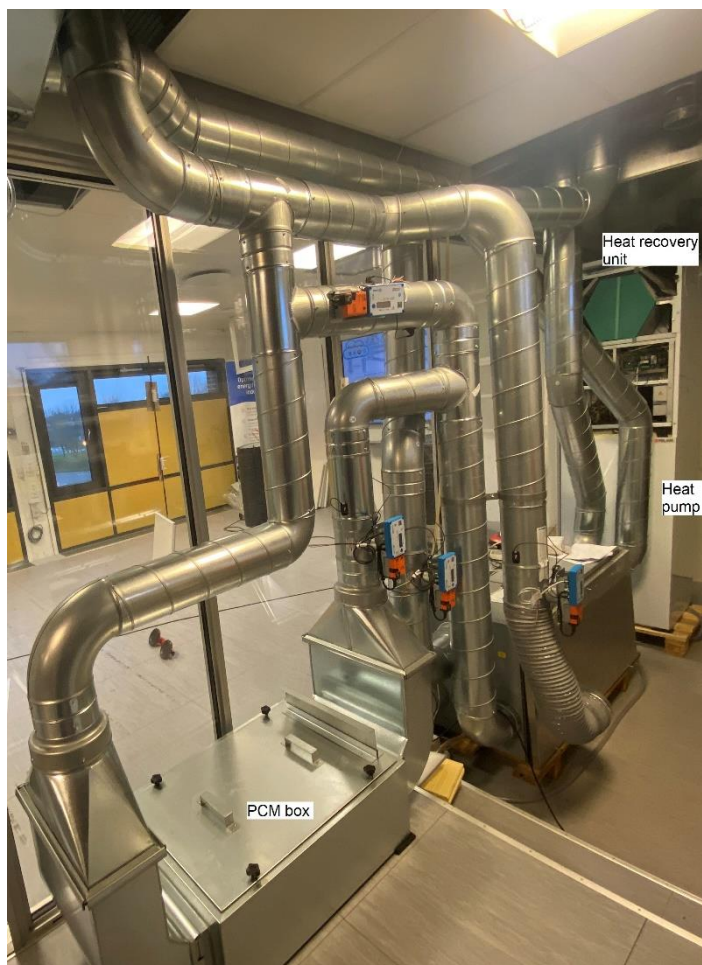
Figure 13: The setup of PCM integrated heat pump system in energy flexibility lab [2].
