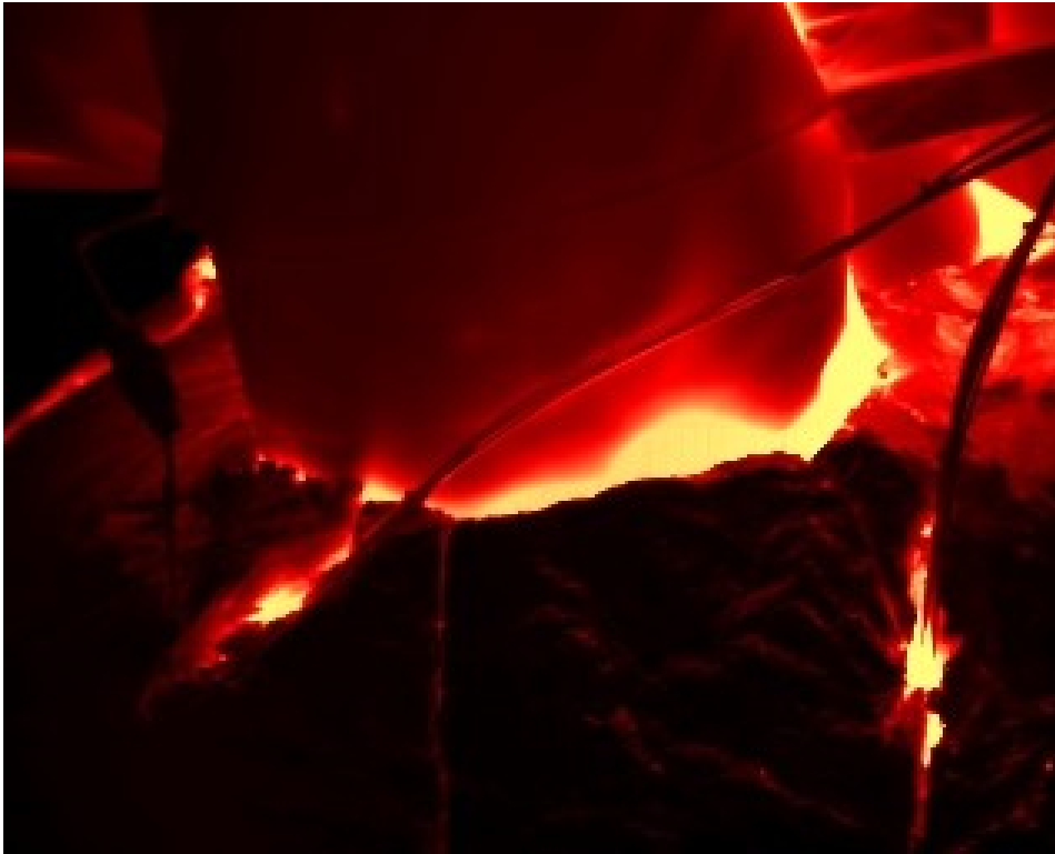
Figure 6. Infrared image of center column surface after 42 hours of charge.
