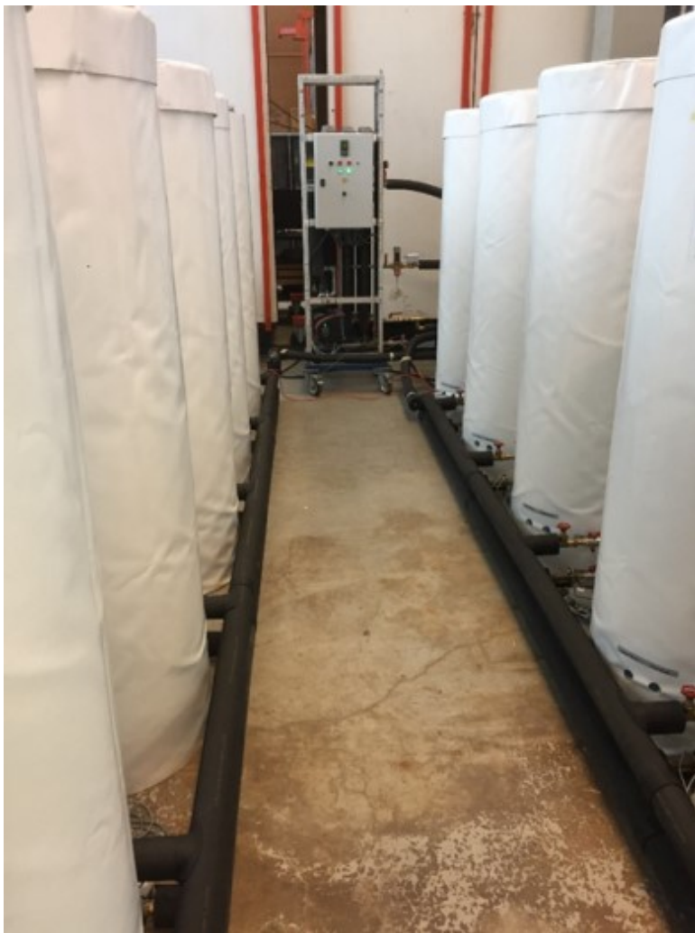
Fig. 15. Modules with PCM from H.M. Heizkörper tested in a laboratory test facility.
