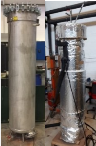
Fig. 5. The PCM heat storage unit with and without insulation.
