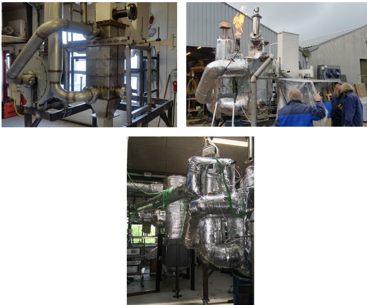
Figure 14. Development of the construction of the updraft pyrolysis reactor at DTU-KT, Campus Risø.
