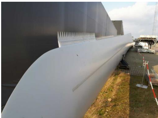
Figure 6 The left photo shows the blade on the ground with the installed FT_008_rev09 and the dino tails (saw teeth elements) mounted on top of the flaps. Later in the autumn 2017 the blade was installed on the 4MW Siemens turbine at Høvsøre – right photo.
