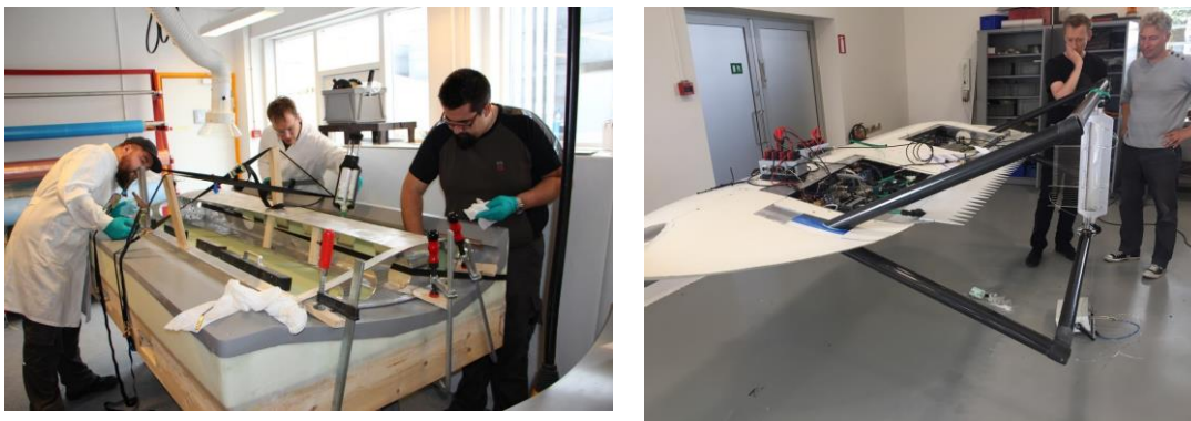
Figure 4 To the left manufacturing of the blade section for the rotating test rig. To the right the blade section has been instrumented. The arrangement with the black poles holds a wake rake that is used for measurement of the drag of the blade section.
