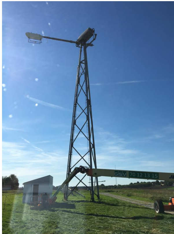
Figure 5 The blade section installed on the rotating test rig test rig.
