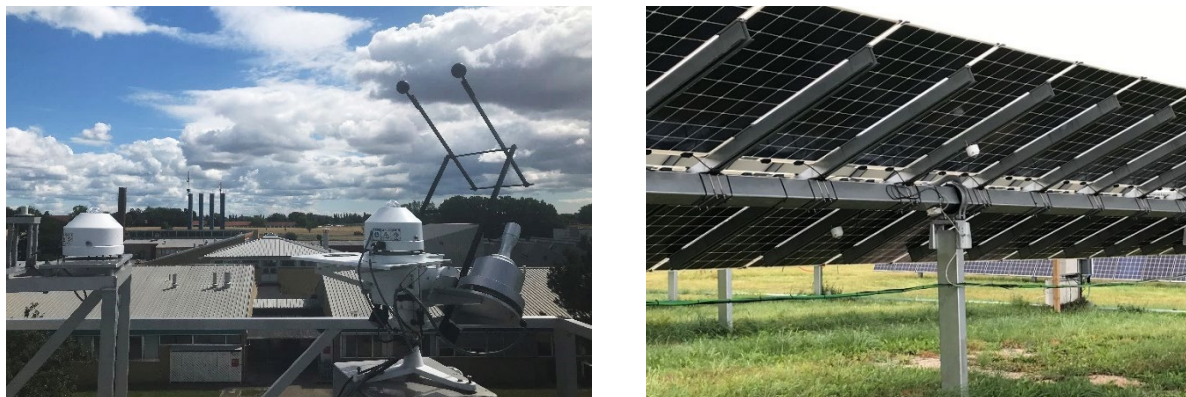
Figure 11: Direct normal, diffuse horizontal, and global horizontal radiation measured at the campus solar radiation monitoring station (left). Spectrally flat class C pyranometers installed on the backside of a fixed tilt array T11 (right).
