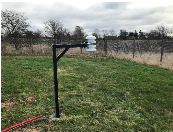
Figure 7 - Spectral albedo setup consisting of an upward and downward facing EKO MS 711 (left) and example data (right)
