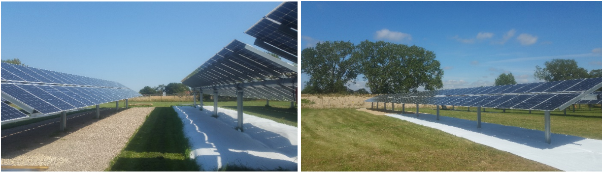
Figure 6 - Ground cover (albedo) experiments on fixed-tilt strings on T10 and T11 (left) and equivalent experiments on HSAT strings on T2 (right)
