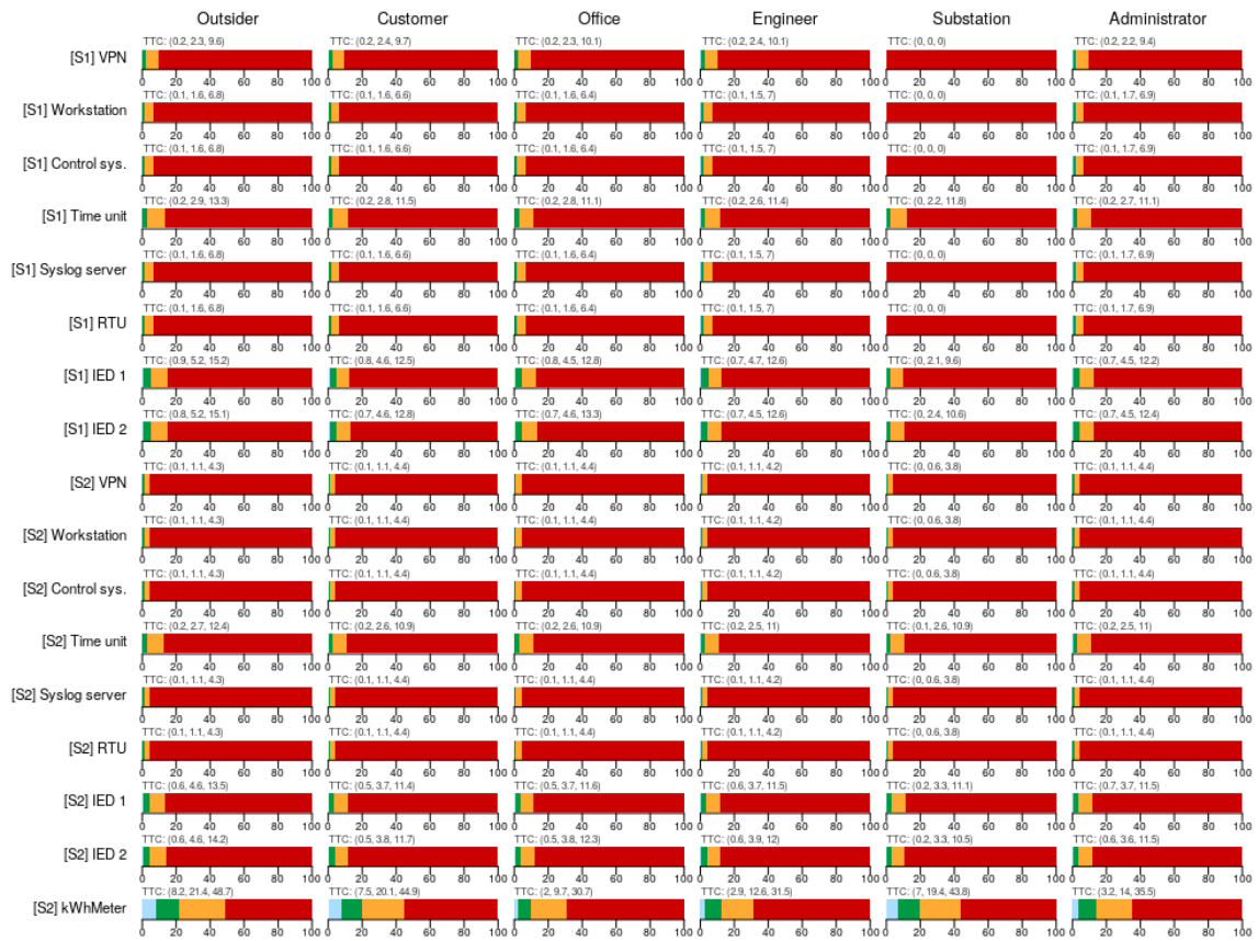
Figure 56: Overview of results from the evaluation of different attacker positions - user access in substation automation.
