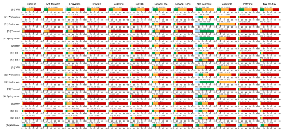
Figure 52: Overview of results from the evaluation of protection scenarios in substation automation - denial of service.
