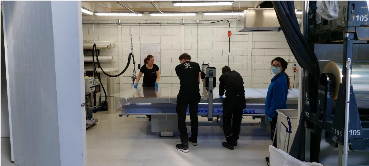
Silicone lens mass production. Glass substrates are placed on a lamination table, silicone resin is dispensed on the glass and the casting film, and a roller is used to distribute the resin over the full glass substrate. After distribution, the resin cures and the lenses are ready for mounting.
