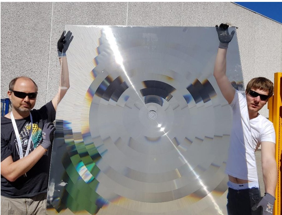
First manufactured silicone lens with the safer lens geometry.
