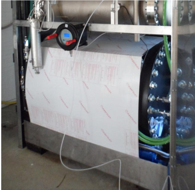
Figure 4: Gas quality sensor being tested and evaluated with the electrolyser in GreenHydrogen's laboratory.
