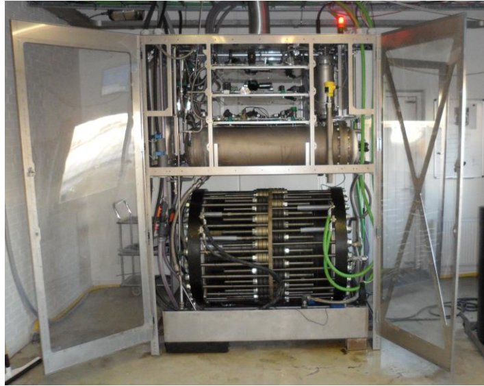
Figure 1. Prototype of a 60 Nm 3 /h alkaline electrolyser unit developed within the project “HyProvide Large-Scale Alkaline Electrolyser (MW)” during the years 2011 to 2015.
