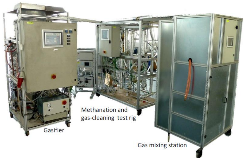
Figure 19 Bench-scale bio-SNG test rig (5 kW fuel) with indirect gasifier. The methanation catalyst operates around 250 °C, 5 bar pressure (Baumhagl, 2014).
