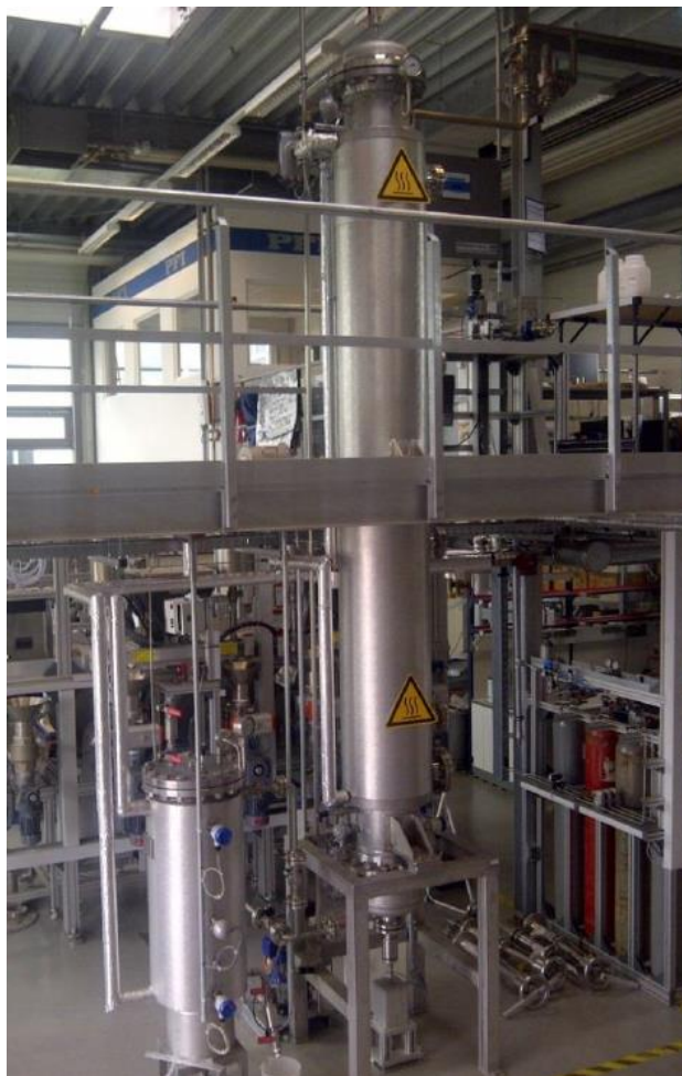
Figure 27 Pressurized, trickle-bed reactor with gas recycle (Dröge, 2016).
