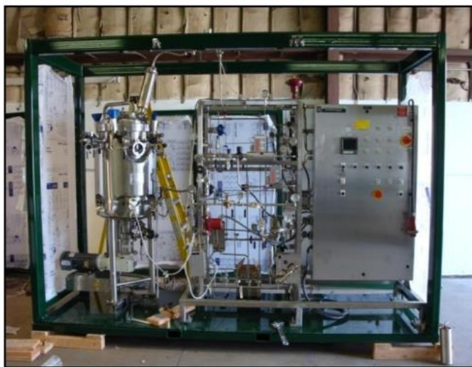
Figure 25 Mobile plant to demonstrate the syngas fermentation of biomass derived syngas (LanzaTech).
