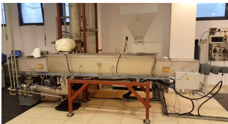
Figure 9 Direct electrically heated auger pyrolysis, capacity 6-60 L/hour, operating at max. 800°C (ETIA, France)
