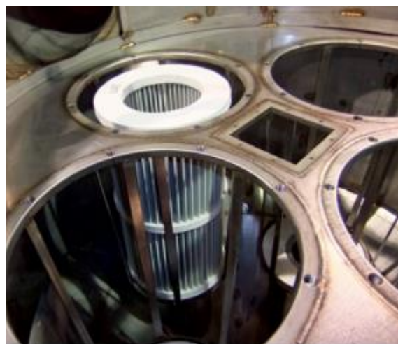
Figure 16 Cartridge filter for small-scale gasifier applications (CerX Ceramic filtration Systems, USA). Available in various lengths and 10" to 30" in diameter.
