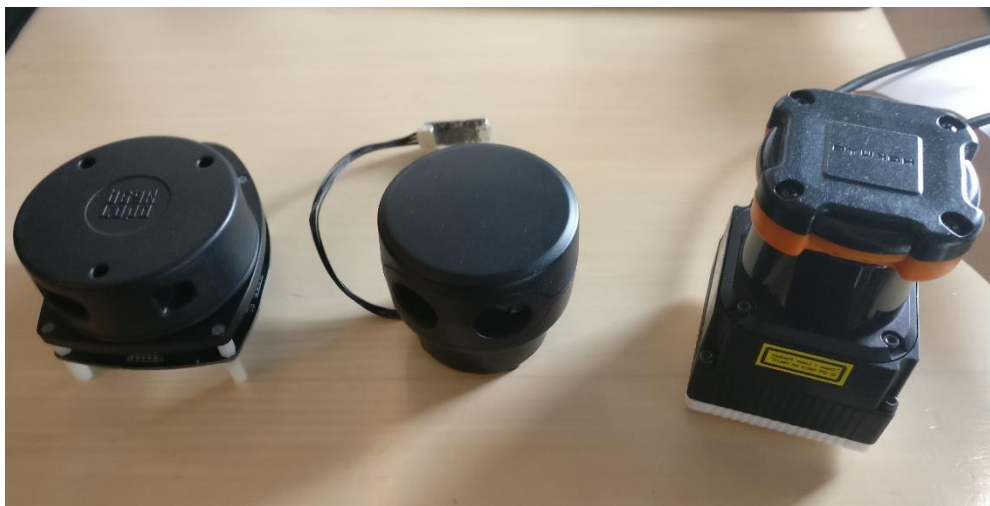
Figure: All the tested LiDAR solutions - from left to right - the rplidar, Scanse Sweep and Hokuyo UTM-30LX
