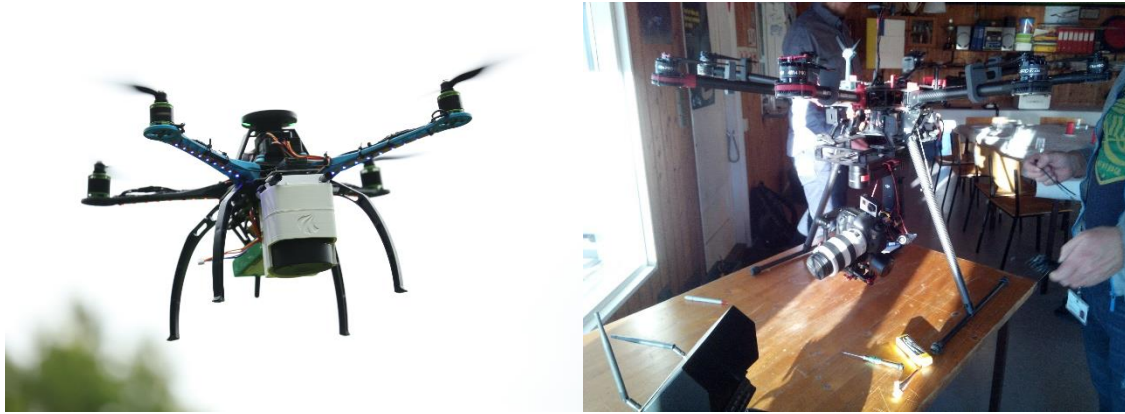
Figure: The Iris+ small drone with the LiDAR attached to it (left) and the DJI S1000 drone with the camera and gimbal attached
