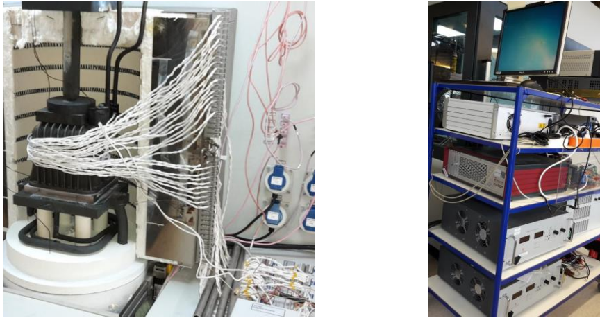
Figure 20. (Left) Photo of mounted TSP-1 stack, with voltage wires. (Right) Photo of transportable EIS trolley
