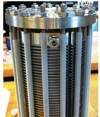
Figure 25. The IRD PEM stack with 33 cells.
