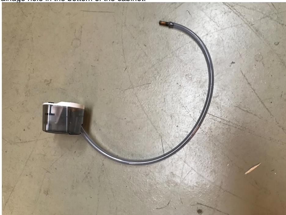
Figure 91 Water collector modified with drain tube.
