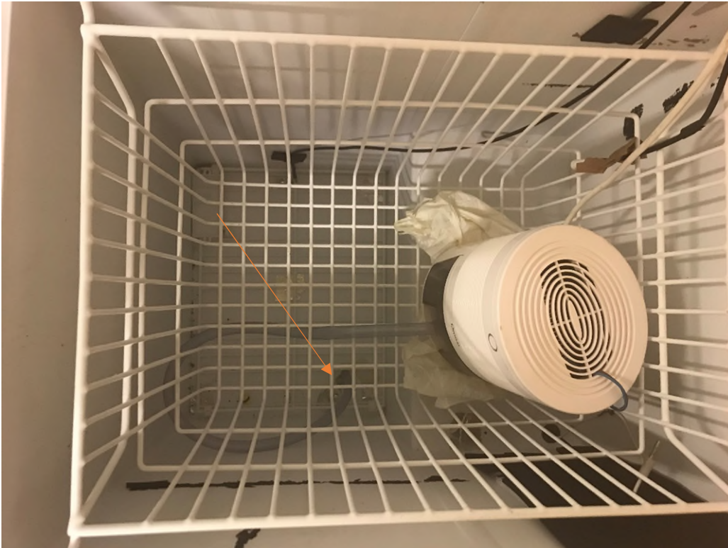
Figure 35: The thermoelectric dehumidifier placed inside the vaccine chamber. Drainage through bottom plug.
