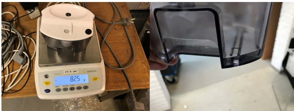
Figure 89 Collected amount of water after one week and without additional humidity load (only some door openings).
