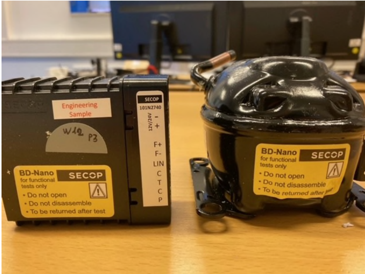
Figure 18: Photo of the prototype BD Nano Compressor (photo by Hendrik Möller, SECOP).
