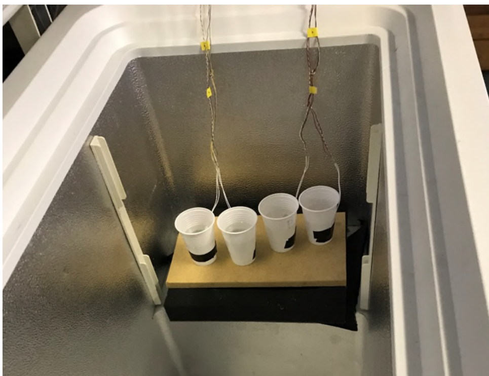
Figure 71 Freezer with water filled cups and various additives. External mounting of sensors. A vibration damping mat was used to avoid vibrations from the compressor that could possibly trigger freezing.
