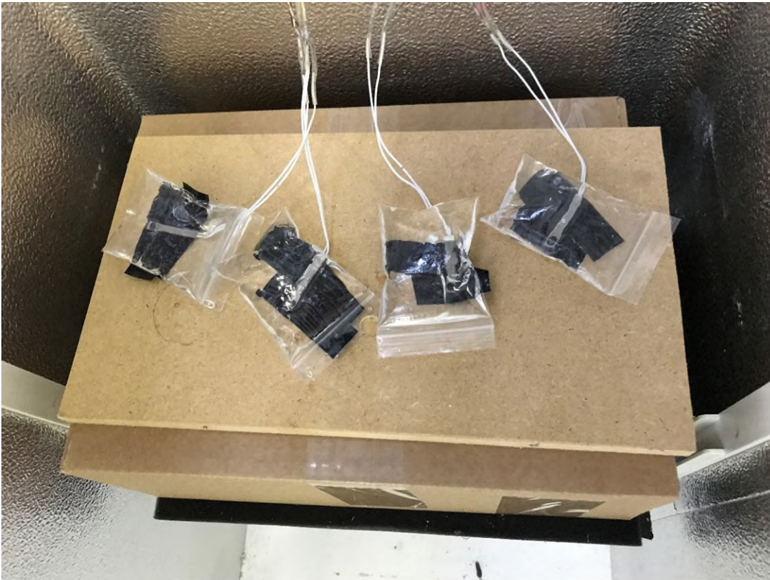
Figure 74 Plastic bags with temperature sensors taped to the lower surface.
