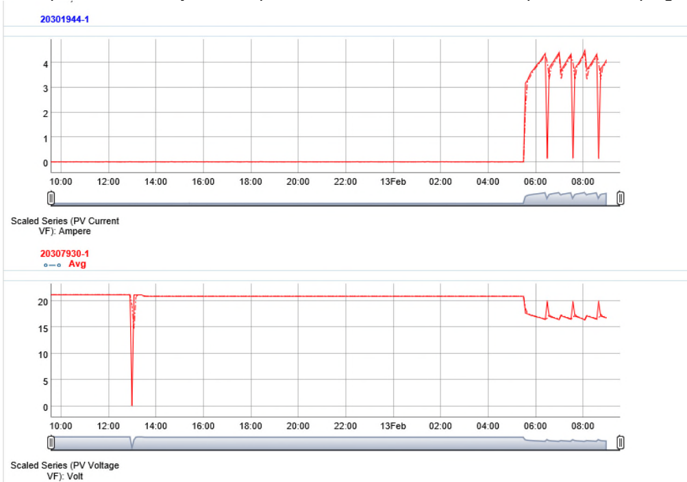
Figure 105 Start and ramping up. Restarting three times because it can't reach full speed.
