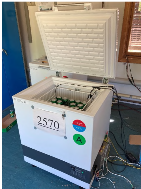
Figure 33: Pull-down test with 50 warm soft drink cans inserted per day. The test was conducted in the “solar house” at DTI in June 2021.
