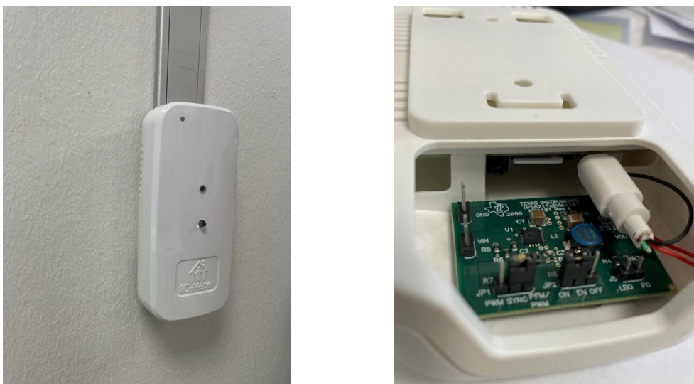
Figure 5: IC meter with power sourcing in Tracy
