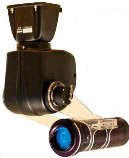
Figure 4 The 3" lidar telescope can be steered by a pan and tilt head
