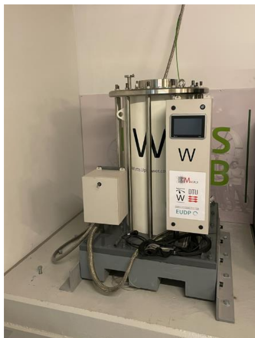
The flywheel delivered by Wattsup to DTU, installed on the foundation made by DTU Elektro.
