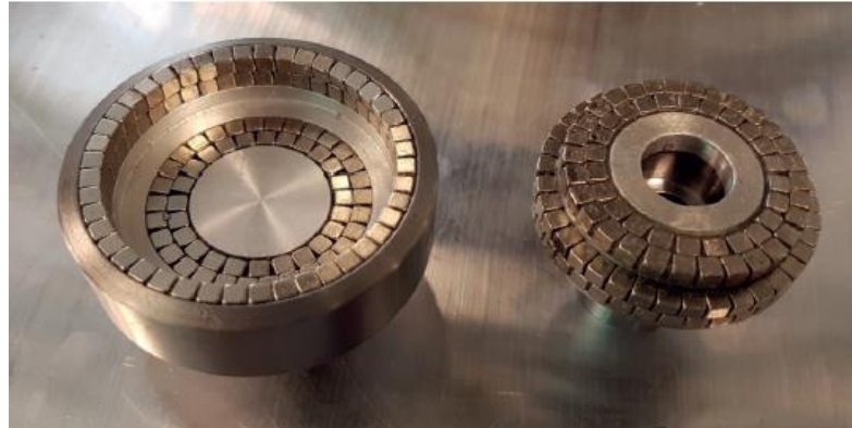
A passive magnetic bearing developed by DTU Energy in the project. The bearing consists of a stator and a rotor part.
