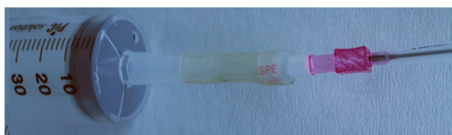
Fig. 4. SPA sampling: needle with cartridge fastened to syringe via rubber band.
