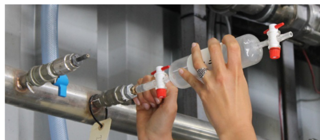
Fig. 5. Gas pipette sampling with rubber tube connection to sampling port.
