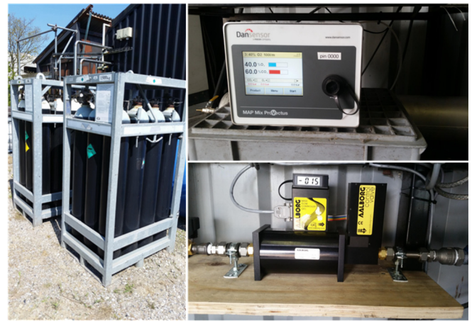
Fig. 3. Experimental setup for converting the air-blown gasifier to O 2 -CO 2 -blown. Left: Gas bottles. Upper right: gas mixer. Lower right: mass flow controller.
