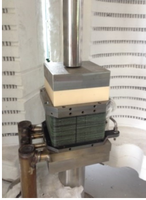
Figure 5 - SOFC stack mounted in oven
