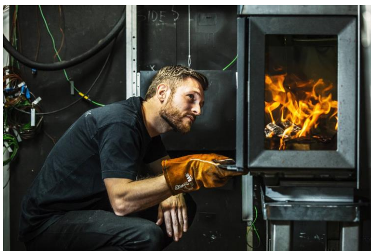
Testing combustion chamber design at a woodstove. (Photo: Danish Technological Institute)
