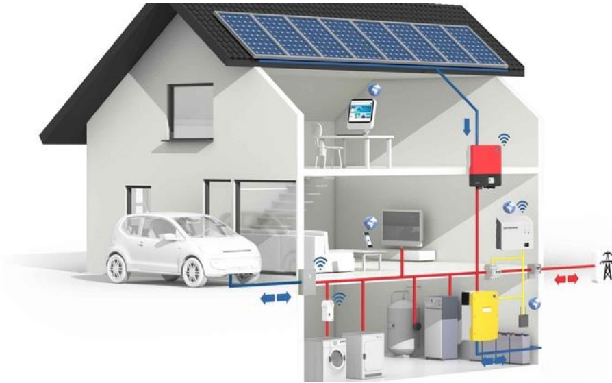
Figure 12: Integration of battery storage, PV system, EV charger etc. Available from SMA inverters.
