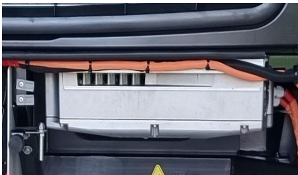
Left: Inverter mounted in the eTRU refrigeration unit. Right inverter prototype PCB
