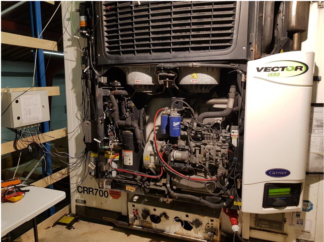
Initial test setup on the diesel driven trailer with extra pressure and temperature sensors mounted.
