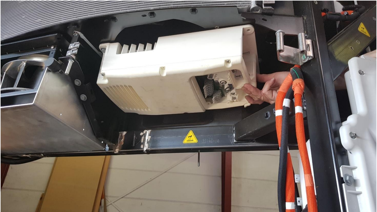
Fit check of prototype inverter to drive the compressor.
