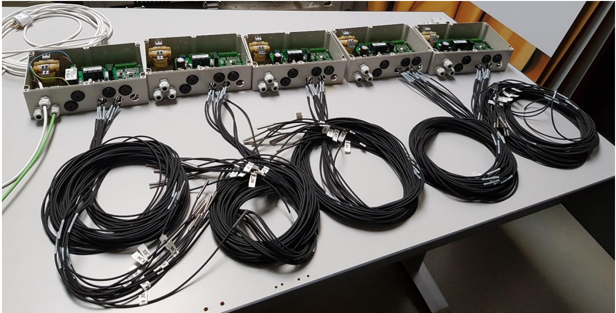
Temperature measurement equipment used to measure air temperature distribution in the trailer. This was used to ensure proper temperature distribution during optimization of the airflow.
