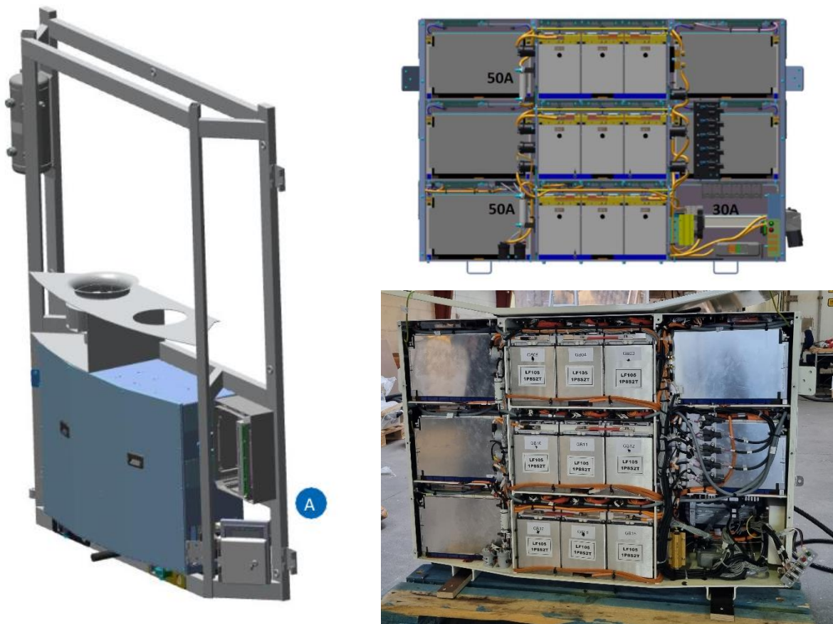
Left: Battery pack in the refrigeration unit frame. Right: topology of battery modules in the pack.
