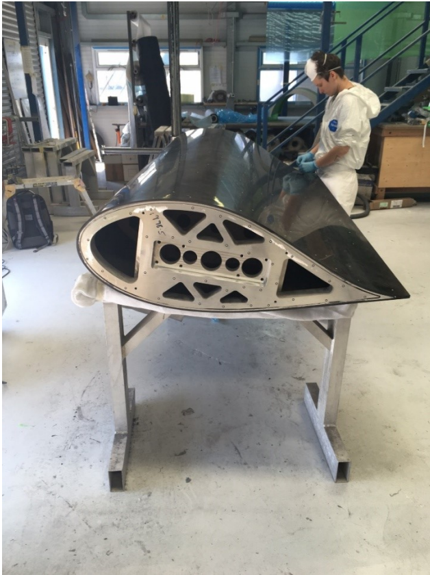
Figure 5: The 35% thick DU airfoil model ordered at Designcraft for the PLC wind tunnel tests
