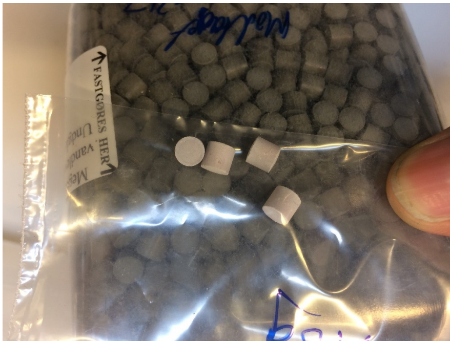
Figure 4. Picture of pellets after regeneration (grey) compared to the non-regenerated pellets (dark grey/black)
