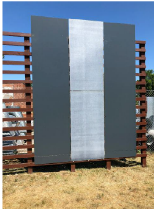
New BIPV technology from Danish Solar Energy, with light grey panels in the middle and with Rock panel façade, was demonstrated by Solarplan, showing PV production quite near normal crystalline PV modules
