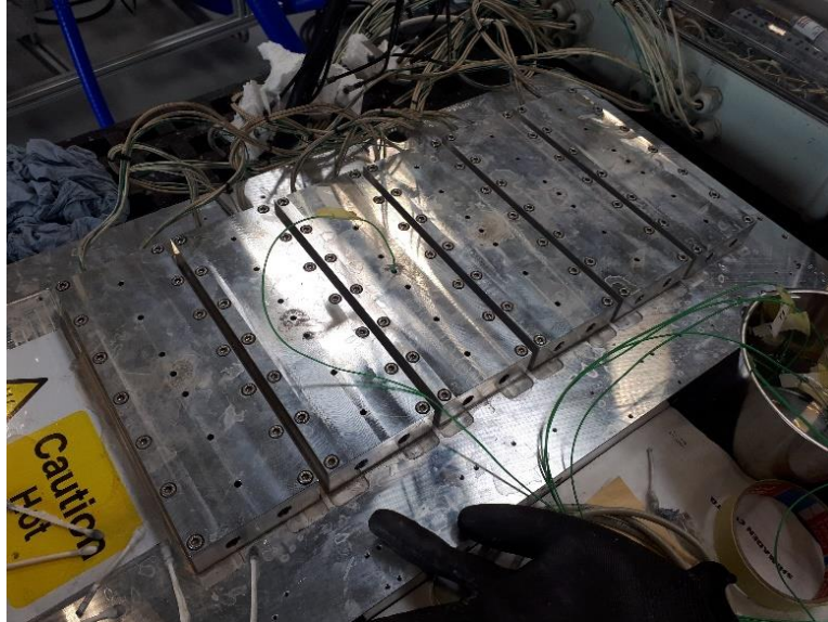
Figure 1 - 6 IGBT mockups mounted on a cold plate in the laboratory.
