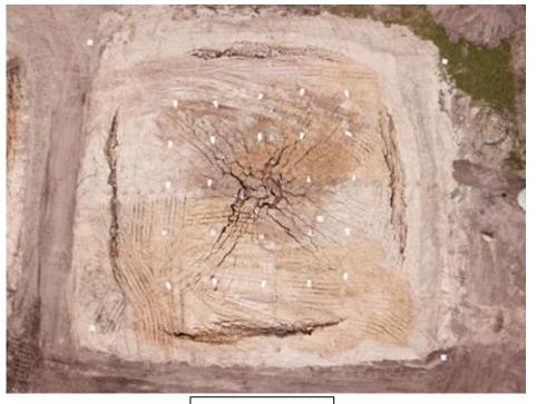
Aerial photo showing peripheral cracks and diagonal cracks.
