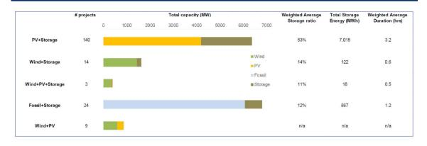
Notes: Not included in the figure are 108 other hybrid / co-located plants with other configurations; details on those plants are provided in the table on slide 7. **Storage ratio** is defined as total storage capacity divided by total generation capacity within a hybrid type. **Duration** is defined as total MWh of storage divided by total MW of storage within a hybrid type.
