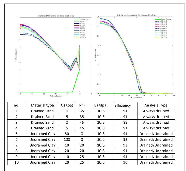
Fig. A2. 17: Sensitivity study in Optum of the effects of soil type on overburden surface and membrane inflated state at full prototype (L100C20D3M1, hill-shaped)
