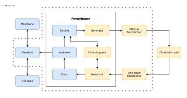
Fig. 3 The dotted line contains the key elements in the hydro electrical system
