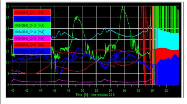
Fig. A4. 17: Output signals in mA (range between 4-20) from selected strain gauges during series . Note the factory calibration is 0.427mA / %volumetric strain.
