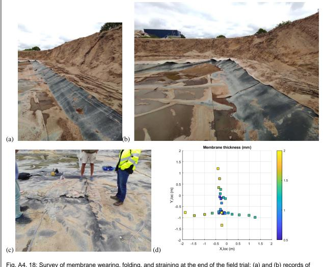
Fig. A4. 18: Survey of membrane wearing, folding, and straining at the end of the field trial: (a) and (b) records of folding at the edge zones. (c) central zone of rupture, (d) measurements of membrane thickness in the central zone post field trial testing.
