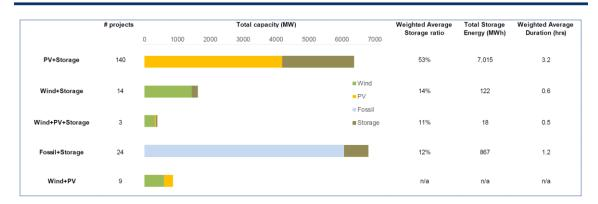
Notes: Not included in the figure are 108 other hybrid / co-located plants with other configurations; details on those plants are provided in the table on slide 7. **Storage ratio** is defined as total storage capacity divided by total generation capacity within a hybrid type. **Duration** is defined as total MWh of storage divided by total MW of storage within a hybrid type.
