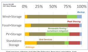
Grid services category includes the following: frequency regulation, load following, ramping/spinning reserve, load management, and voltage/reactive power support
