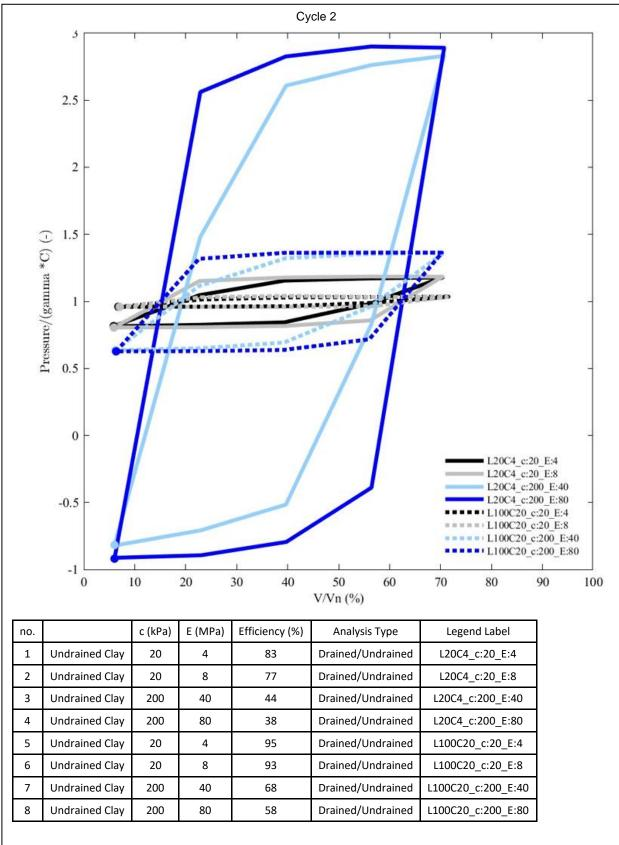
Fig. A2. 20: Optum modelling results of the effects of clay strength and stiffness parameters on energy performance on full prototype (hill shaped; L20C4D0.6 and L100C20D3)
