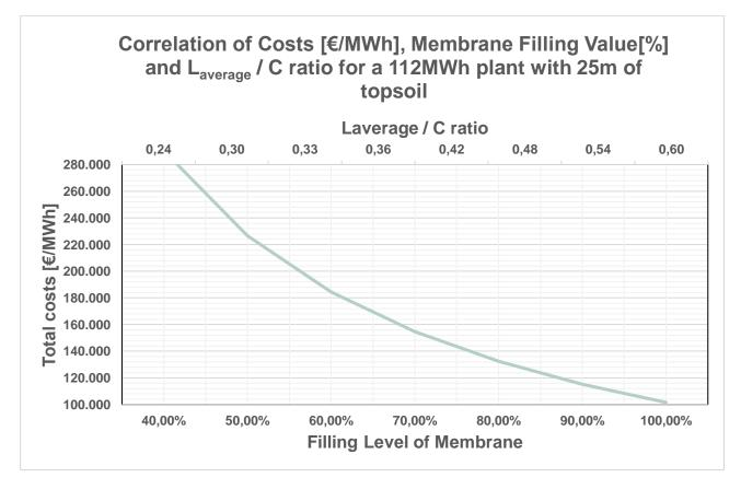
Fig. 11 A total price relation with  $L_{average}$  / C ratio and Filling Level of Membrane.
