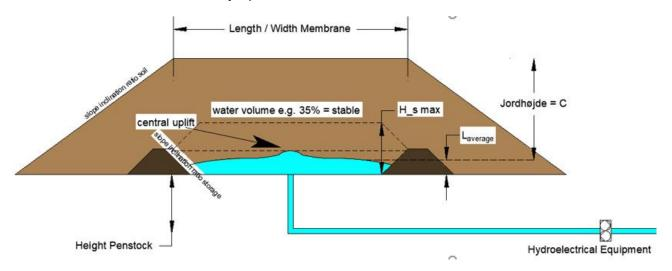
Fig 1 Figure containing the key measures of a "standard" one unit membrane system. Key annotation of the different measures has been indicated. Also, we see the indication of the potential limitation of the lifting height.
