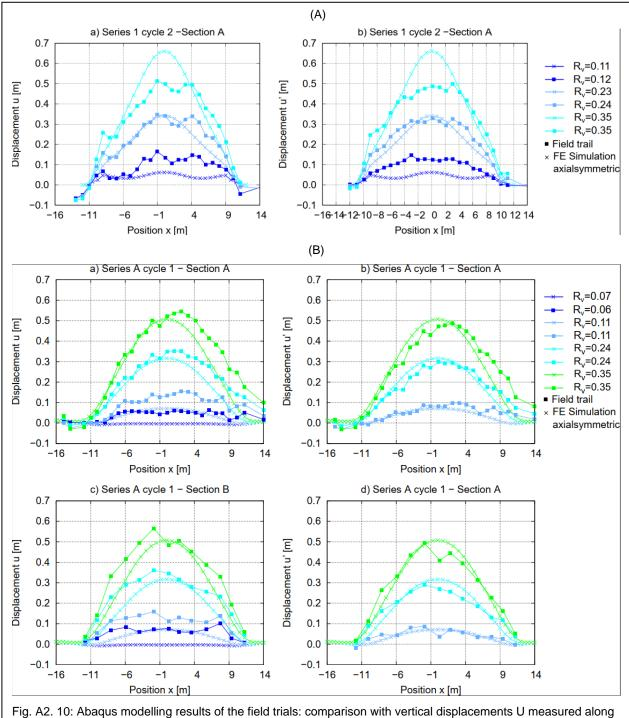
transverse section A during the 1<sup>st</sup> cycle of the field trial (A) FT\_C2 with 2m cover and (B) FT\_C2 with 4m cover.
