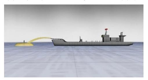
Fig 2. Illustration of an "off-shore" version of the an UPHS system. Turbine needs to be made of non-corrosive materials as it will be saltwater running through the system
