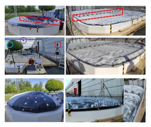
Fig. A4.3: Square and circular reservoir alone testing: (top) deflated configurations with highlighted transverse section being monitored; (centre-left) monitoring set-up; (centre-right) partly inflated state of the square membrane with associated folding; (bottom) fully inflate state of the reservoirs.
