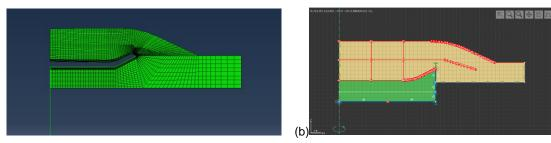
Figure 1 Geometries of the (a) refined Abaqus and (b) simplified Optum UPHS models for the preliminary geometry **PR\_C4**.
