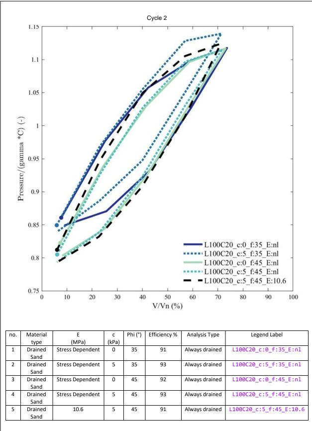
Fig. A2. 19: Optum modelling results of the effects of sand strength parameters on energy performance on full prototype (hill shaped; L100C20D3 , ie 5times FT\_C4 )
