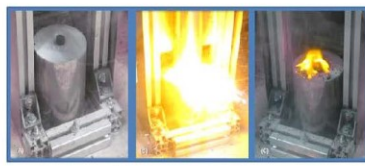
Fig. 2. A 4-gram NaAlH 4 wafer ignited upon first impact (free fall height = 1 m).
