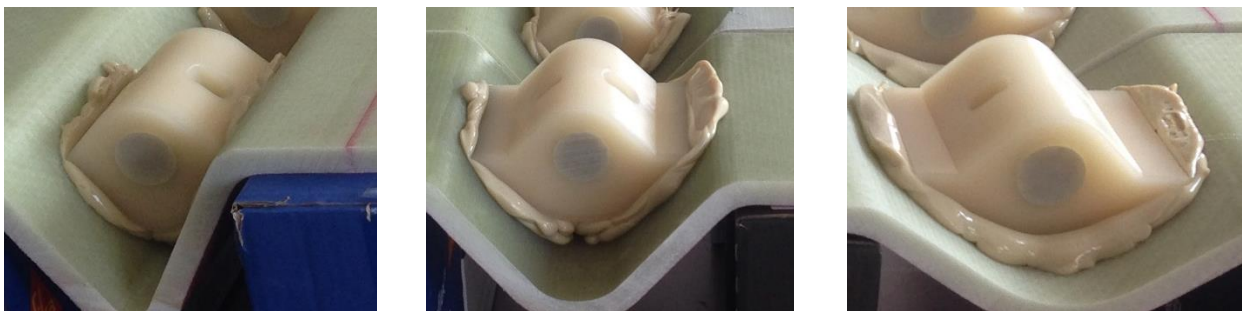
Figure 24 – Photo showing the 3 different corner mounts produced to cover angles between 60° & 140°
