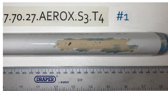
Figure 122 - Specimens after 2 hours in RET. Large zone eroded.
