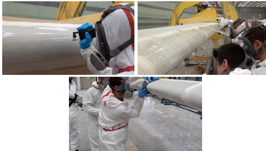
Figure 41 - Application methodologies on wind blades. Left: spray. Centre: roller. Right: filling knife.
