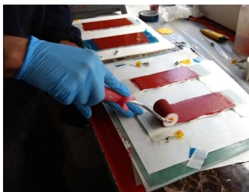
Figure 32 - Incorporation of TNO sensor fibres in Aerox coatings at Aerox laboratories (Valencia, Spain).
