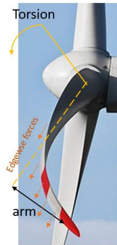
Figure 109 - Torsional moment created by the twisting of blade when the blade is subjected to combined loading.
