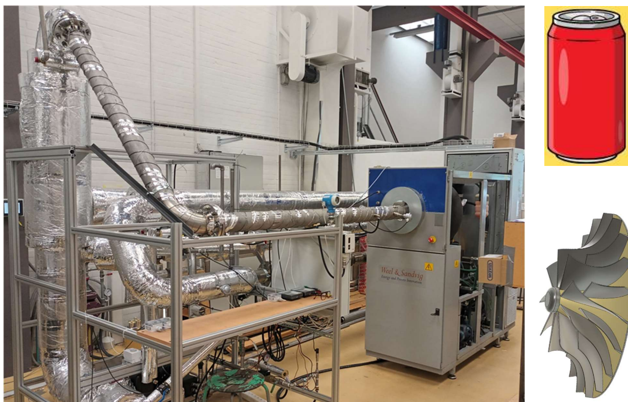
Figure 6. Left: Test rig and compressor unit as built and installed at DTU lab. Lower right: turbo compressor impeller (outer diameter 142 mm) capable of delivering 1 MW condensing heat at 133 C with a temperature lift of 25 C at a rotational speed of 70000 rpm. Upper right: For comparison of impeller size: the size of a normal beverage can.
