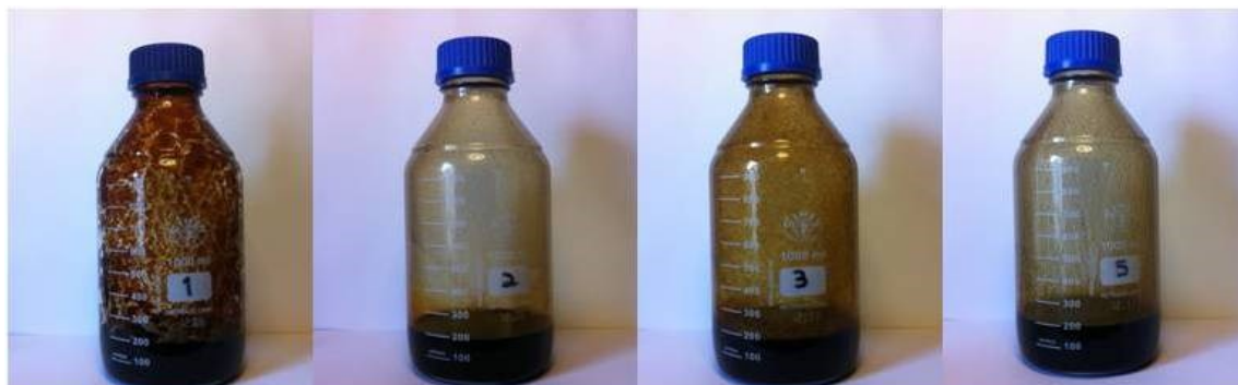
Picture 2.2: 1: Bio oil / Ethanol - 2: isopropyl alcohol - 3(4): Rapeseed oil - 5: RME
