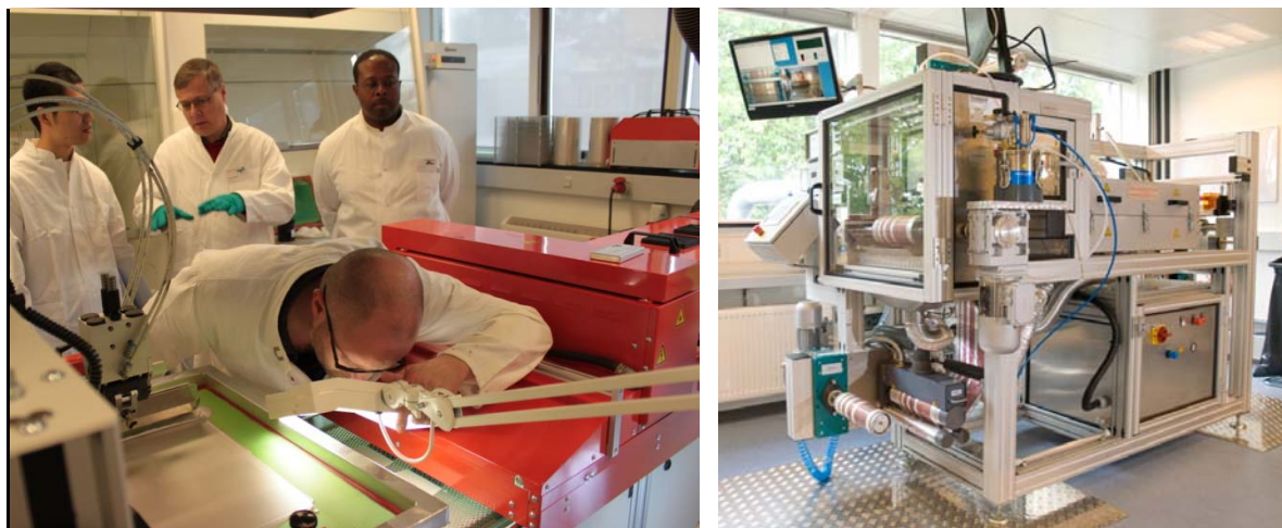
Figure 8: Existing roll-to-roll flat-bed screen printer and roll-to-roll slot-die coater
