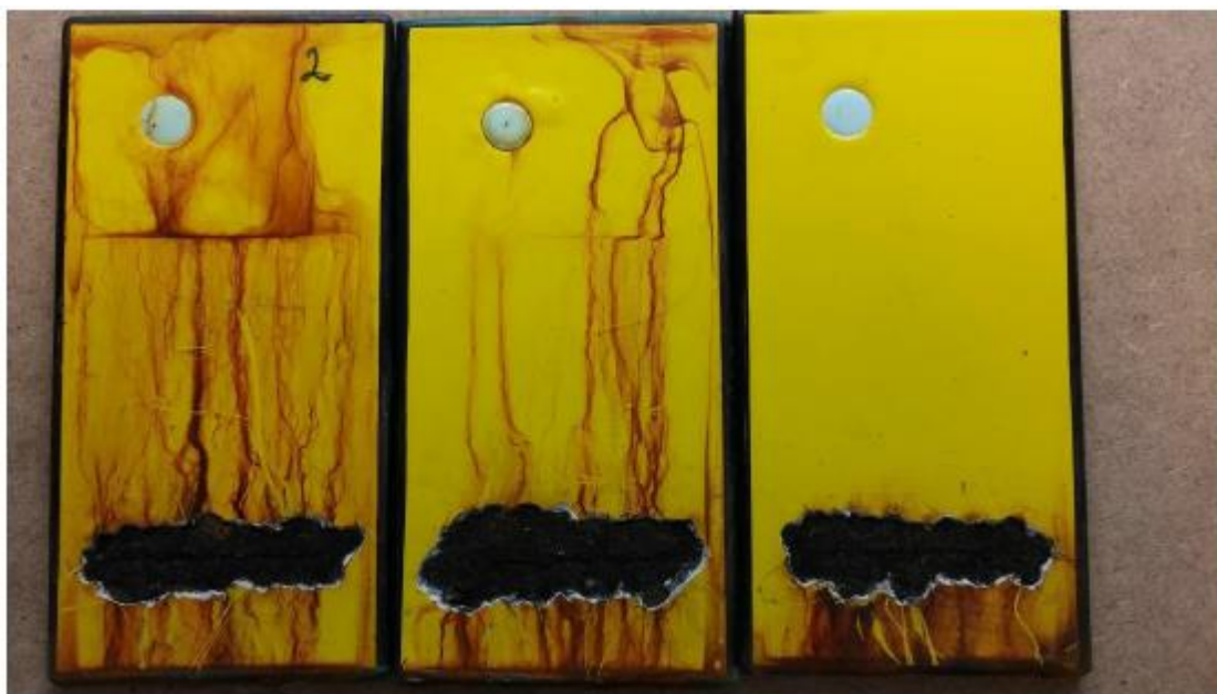
Figure 36 Example of test plate after paint removal
