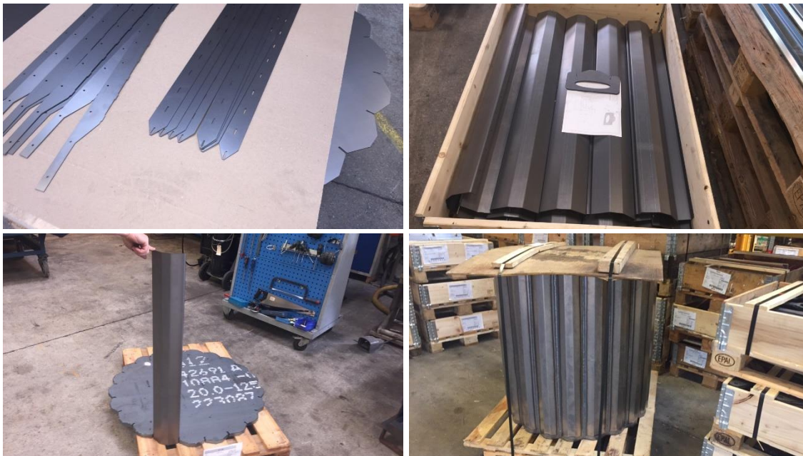
Figure 13 Pieces for the 1m prototype. Upper left: T-stiffeners. Upper right: skirt pieces. Lower left: assembly of skirt. Lower right: fully assembled prototype.
