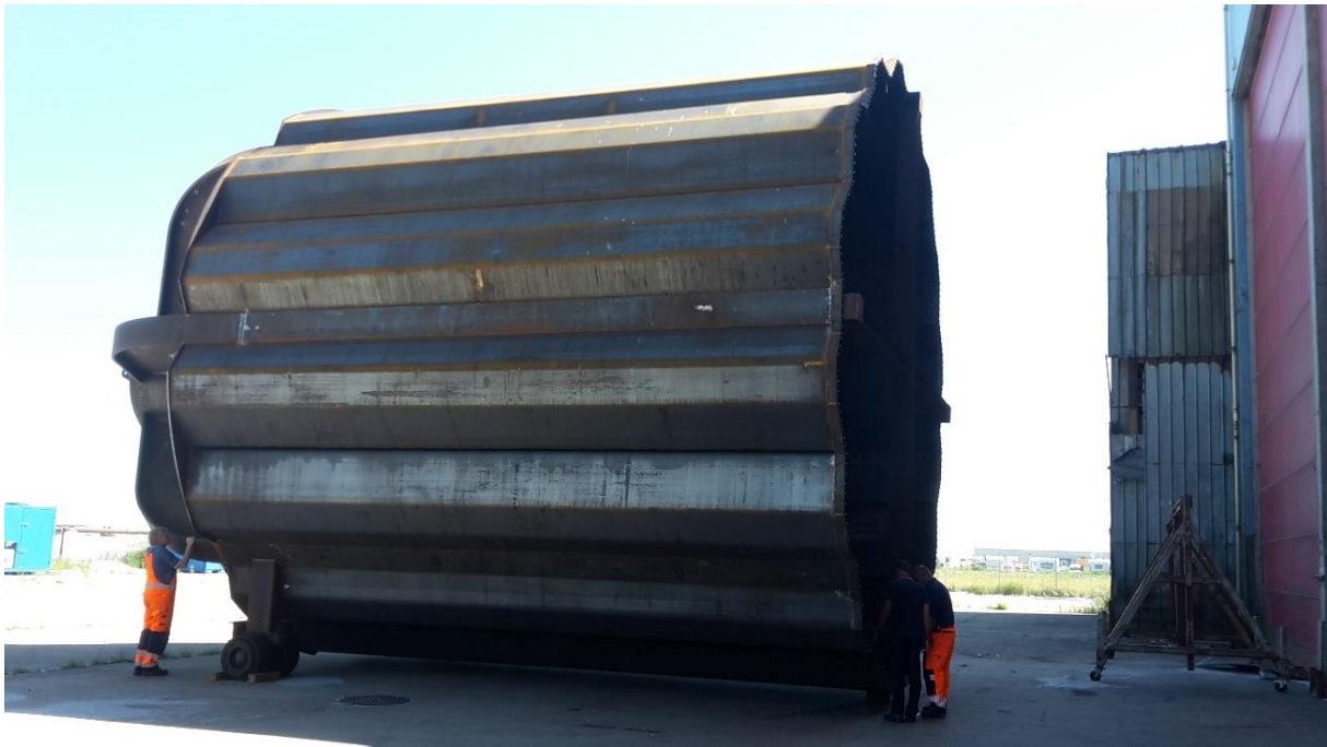
Figure 24 Fully assembled suction bucket
