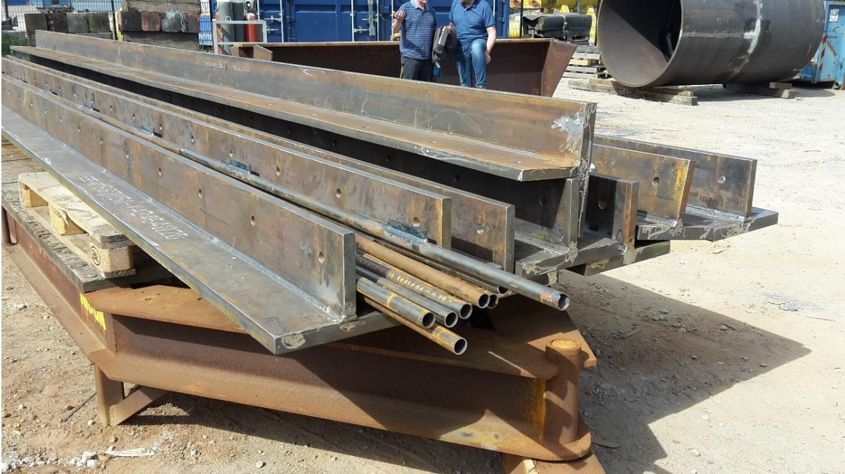
Figure 17 T-stiffeners and flushing pipes
