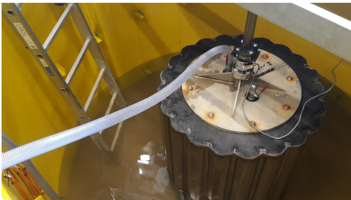
Figure 15 Scale test with prototype modular bucket in pressure tank
