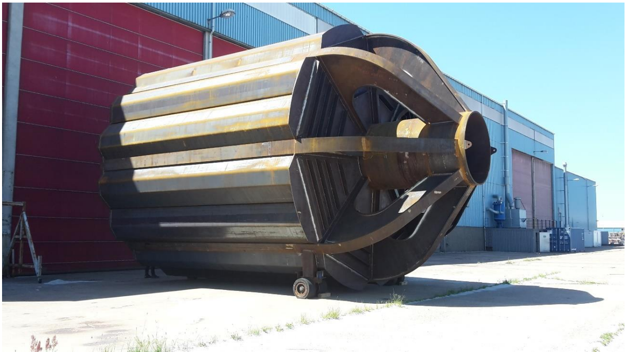
Figure 21 Fully assembled suction bucket
