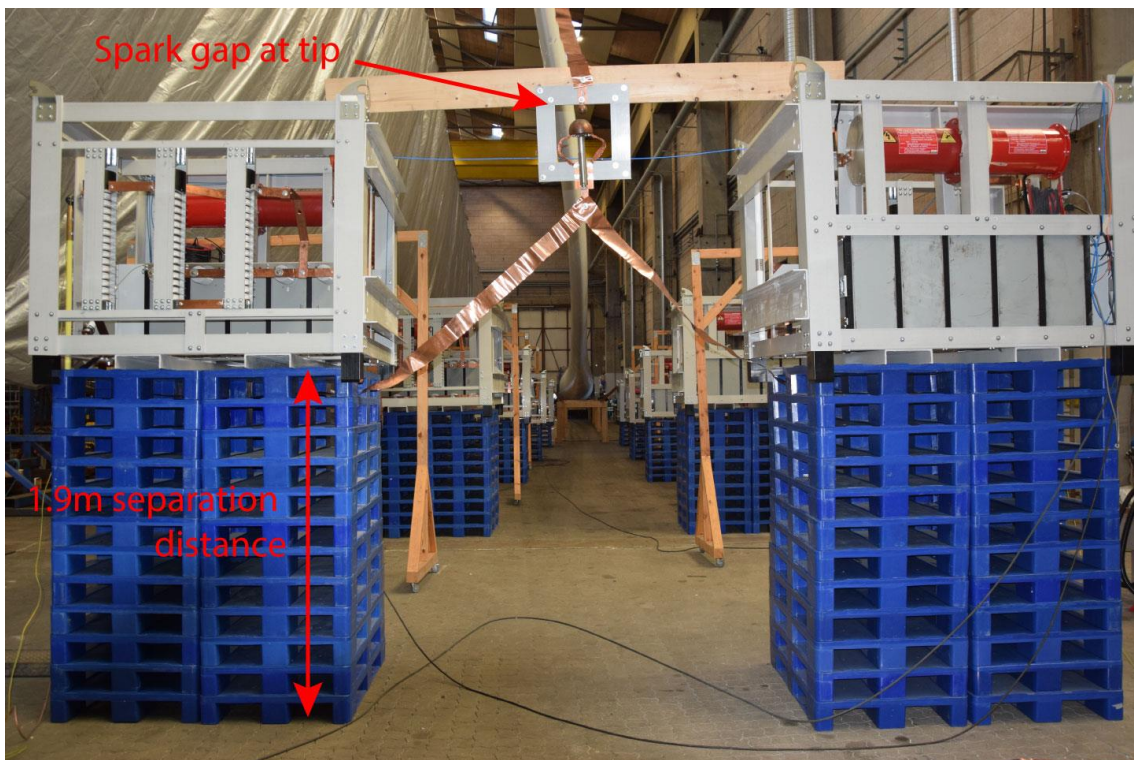
Figure 14 – Photograph from the tip towards the root with the connected ELITE generator (A-bank)
