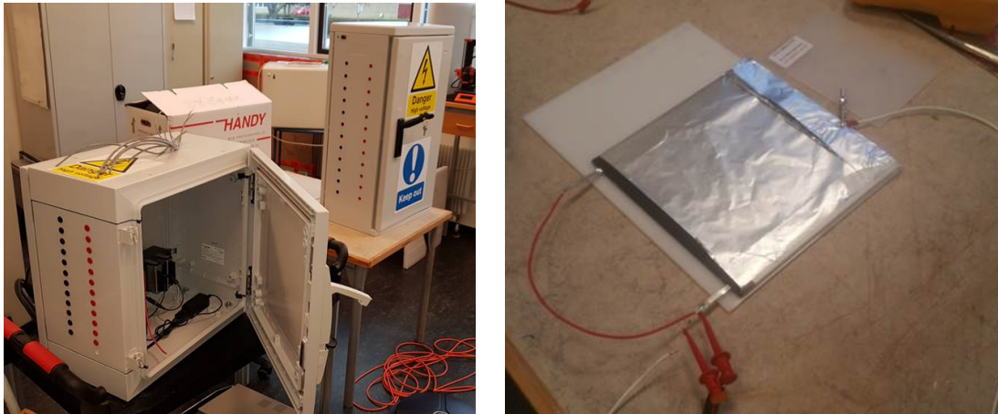
Fig. 17: Enclosures for high voltage power supply, sensing resistors, and test samples (left). Example of test sample wrapped in conductive foil to activate leakage current (right).
