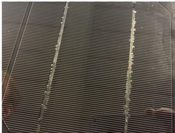
Fig. 3: Laminated solar cells with NiZnS coated ribbons.
