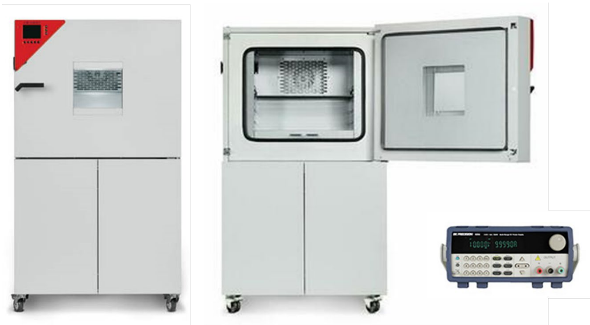
Fig. 23: Thermal cycling test bench at DTU Fotonik.
