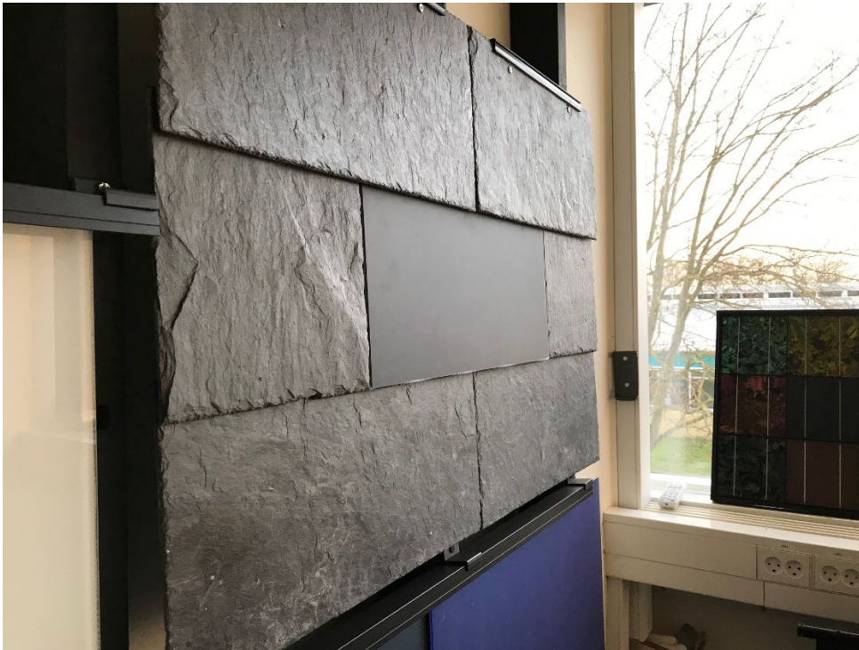
Fig. 24. Solar panel with ADE treated solar cells at NinesPV and selectively dyed strings.
