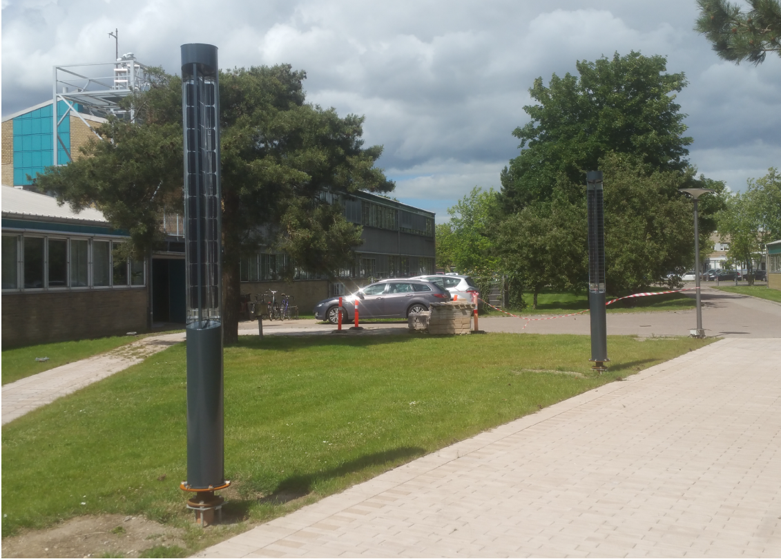
Figure 11: The curved mirror (foreground) and linear mirror (background) reflector columns in DTU Fotonik's Living Lab. The Solar Resource Monitoring Station is in the tower in the top left of the photo.
